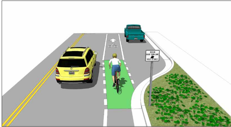
Example of a colored bicycle lane at high conflict areas with motor vehicles. Photo credit: Michael Johnston
